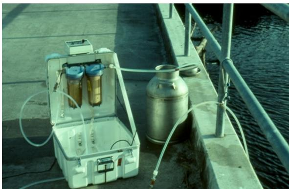
**Figure 13** Portable field-filtration assembly for sampling DOM
