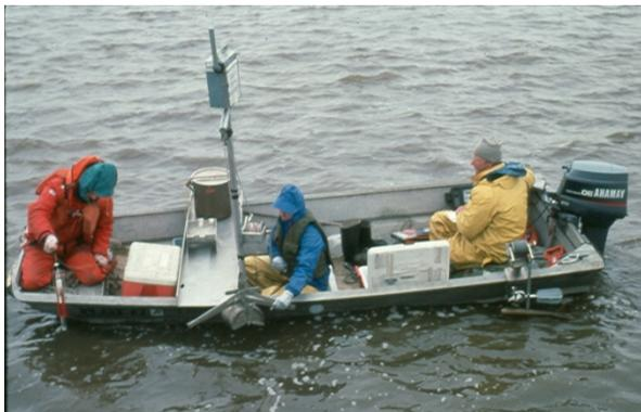
**Figure 12** Sampling bed sediment in a navigation pool in the Upper Mississippi River
