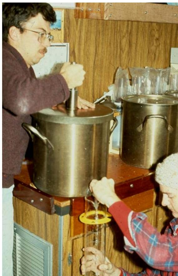
**Figure 11** Sub-sampling depth-integrated water and sediment samples from the Mississippi River with a churn splitter
