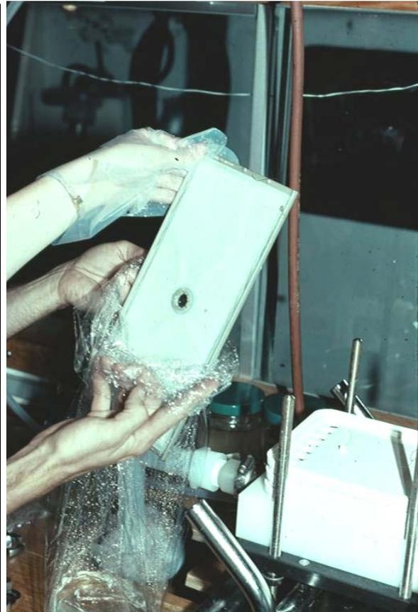
**Figure 9** Placing an ultrafilter plate inside the Teflon bag containing retentate water for removal of colloids that adhered to the ultrafilter membrane
