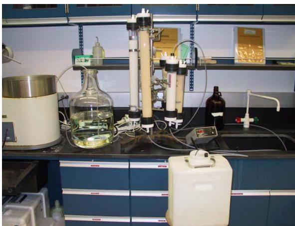
**Figure 14** Polyethylene and glass carboys used as DOM sample containers
