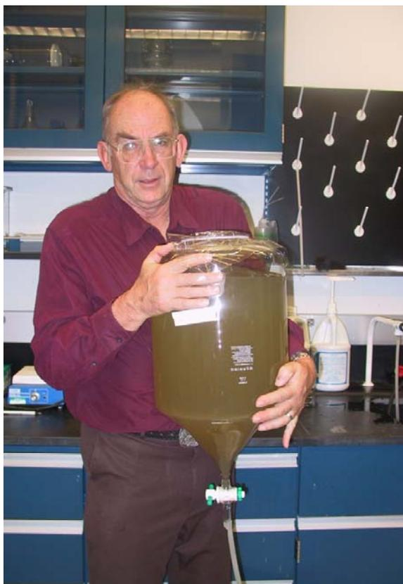
**Figure 64** Stormflow sample from an urban drain into the Santa Ana River; sample is contained in a separatory funnel used to separate sediment NOM from dissolved and colloidal NOM
