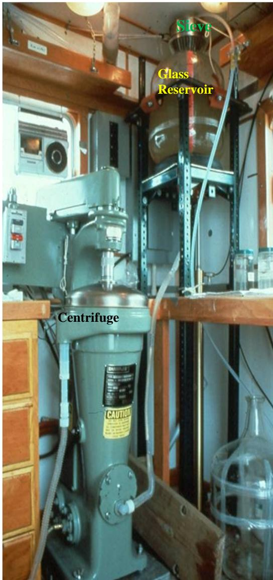
**Figure 6** Centrifuge, sieve, and reservoirs used to process pumped-water sample in the laboratory on R/V *Acadiana*
